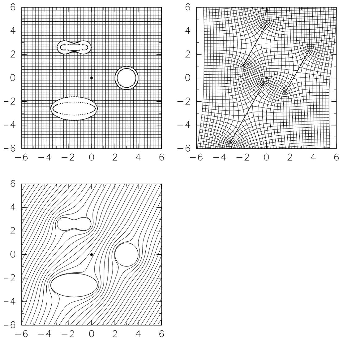
Numerical conformal mapping  $w = F(z)$  and a uniform potential flow i.e.,  $\text{Im}(e^{-i\theta} F(z)) = \text{const.}$
