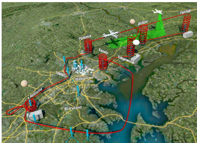
Figure 5. DISCOVER-AQ fourteen day observing strategy for July 2013 over the Baltimore, MD/Beltsville, MD/Washington, DC area. The aircraft ground track has been overlaid on a map of the region showing major roadways. The vertical spirals represent locations where aircraft made descents to measure atmospheric constituents at different levels—to construct profiles. Ground stations are indicated by the towers. Image credit: Timothy Marvel [NASA's Langley Research Center]
